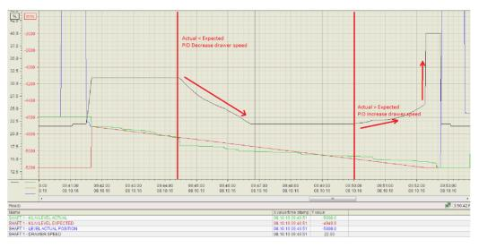
Figure 4 Typical discharge system PID cycle
