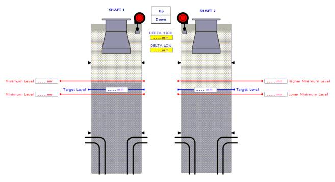
Figure 1 Kiln level representation in a vertical PFR Kiln
