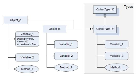
Figure 7 OPC UA representation of an object
