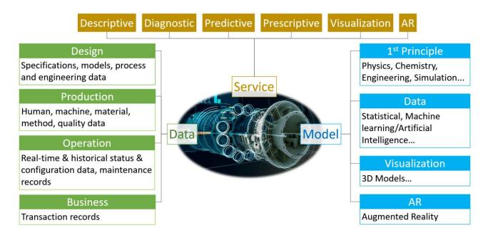
Figure 1: Designing a Digital Twin (Yo-i Information Technology)<sup>2</sup>
