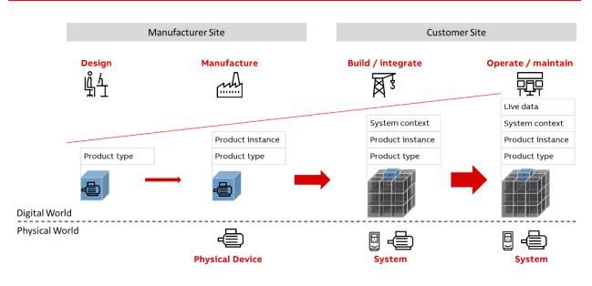
Figure 5: How Digital Twins can tackle the Information Silo Problem (ABB)
