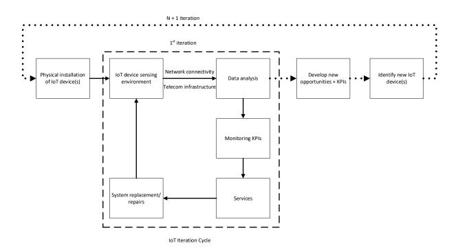
Fig. 16: IoT Iteration Cycle
