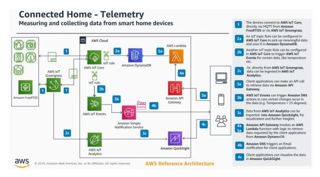
Fig. 15: AWS Telemetry Architecture<sup>64</sup>
