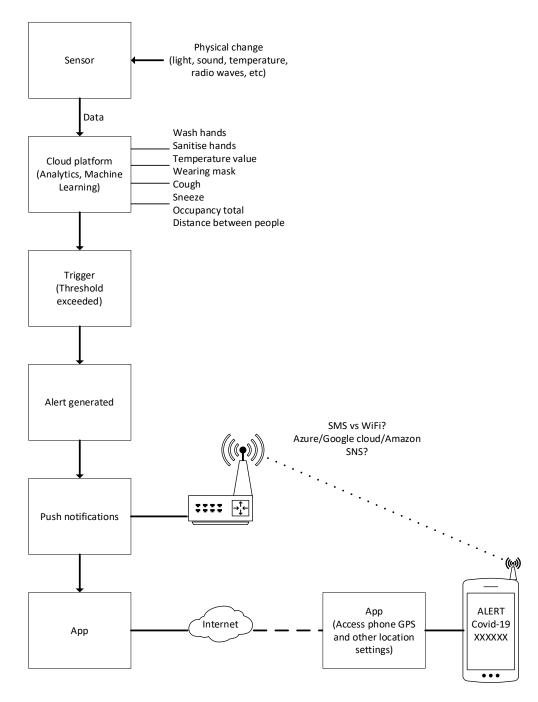
Fig. 14: Conceptual Framework of IoT based Alert System
