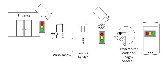
Fig. 12: IoT sensors - External mounted camera, microphone and status indicator
