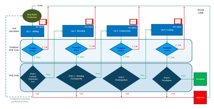
Fig. 5: Tablet Formulation Manufacturing with streaming analytics and predictive analytics
