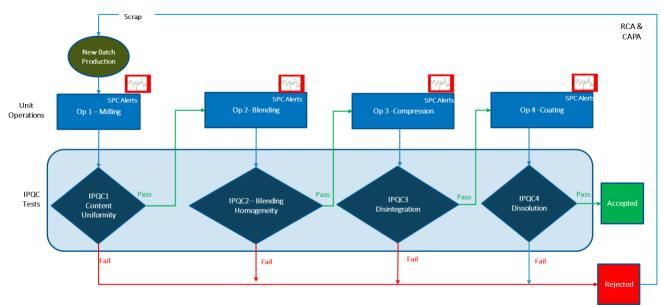
*Fig. 4: Tablet Formulation Manufacturing with standard SPC*
