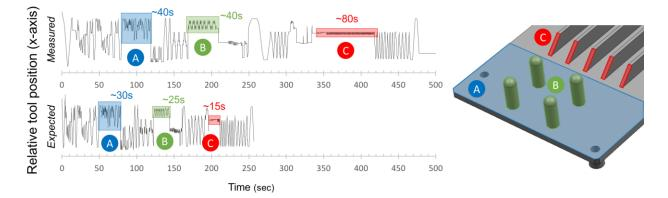
*Figure 3: Comparison of simulated data for part build generated by Mastercam compared to actual machine data. Note: The X-position of each dataset has been translated for ease of comparison. The vertical scales are consistent with both datasets.*
