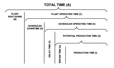
Figure 5: Chart of Equipment Availability Parameters
