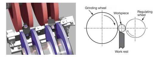
Figure 7: Centerless Grinding
