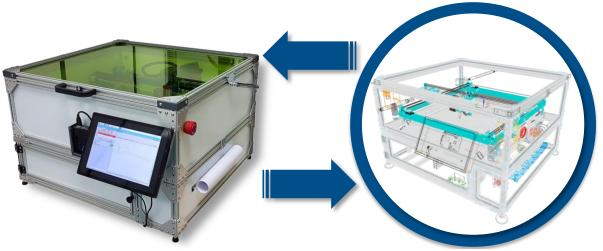
*Fig. 1: Computer-controlled laser plotter as physical asset and the symbol of its web-based digital twin.*
