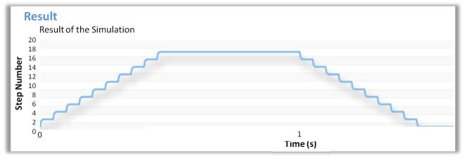
*Fig. 13: Simulation results of an FMU stepper motor simulation on an external simulation server.*
