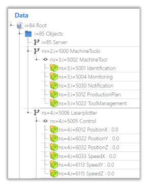
Fig. 9: OPC UA data structure of the laser plotter integrated into the web-based digital twin (ns – namespace, i – Identifier).
