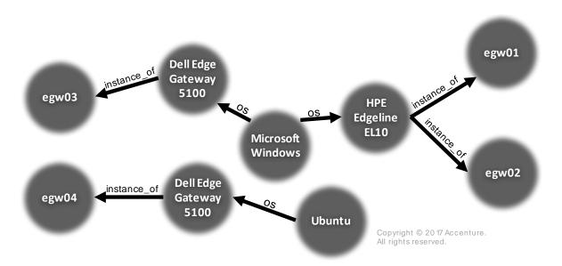
Figure 2: Small section of a client knowledge graph showing HW, OS, and physical gateway instance. Depicts four edge gateways (egw01-egw04) and their HW and OS types.
