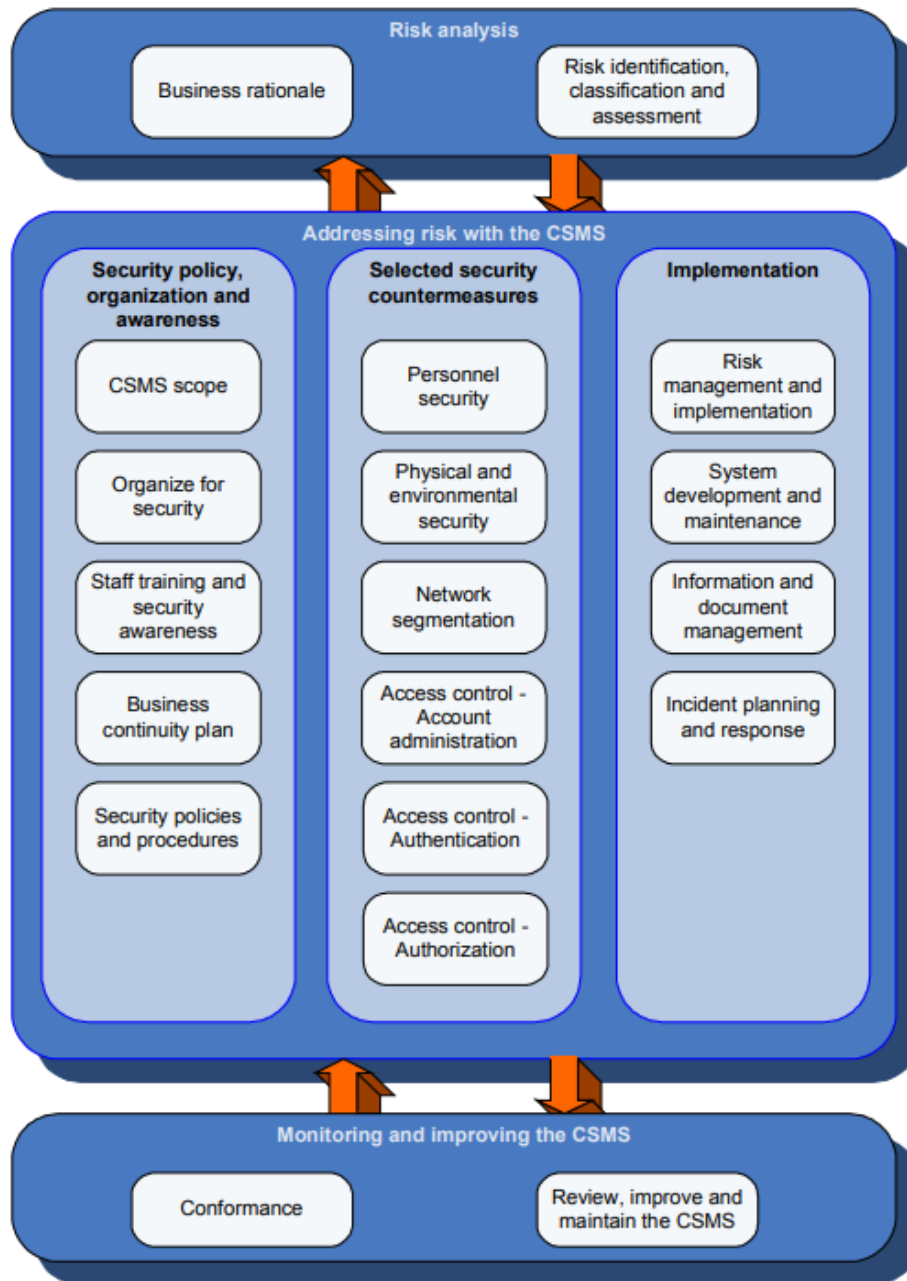
Figure 3-1: Graphical view of elements of a security program (cyber security management system).
